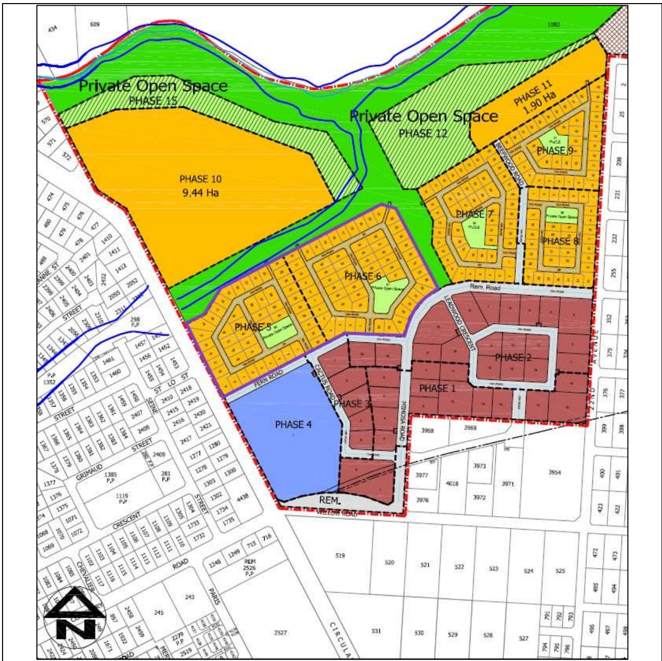
Figure 5.2: Locality map indicating Phase 5 and 6 (purple outline; Residential 2 zoning), in relation to the 1:100-year floodline (blue outline).
